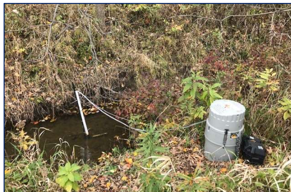
Figure 1- Autosampler, suction line, bubbler line, installed in the Branch & Derby Drain.
