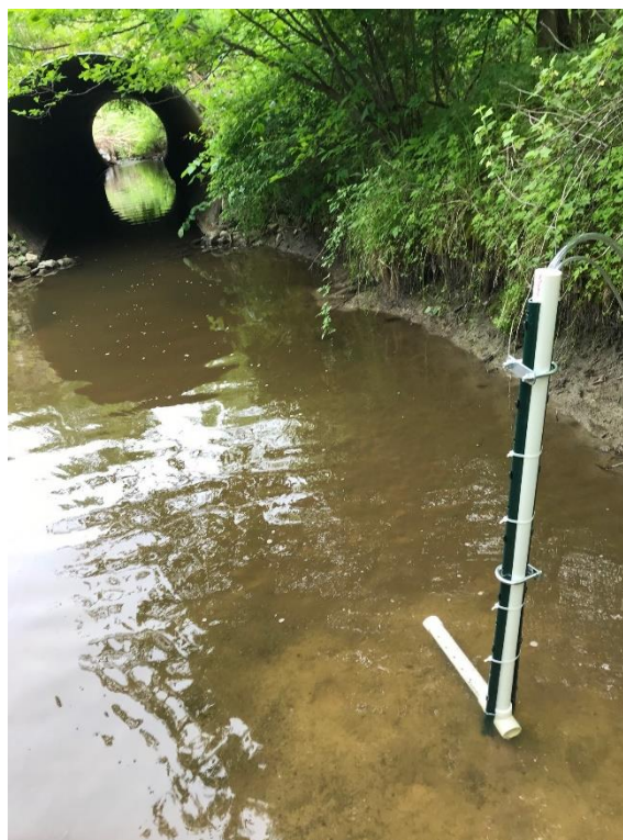
Figure 7 - Autosampler suction and bubbler lines installed on the Branch & Derby Drain, sample site A2, May 2021.
